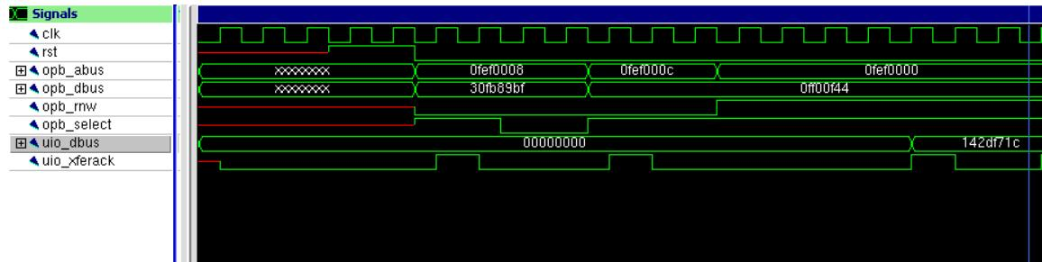
As can be seen, the result is latched to the output only seven cycles after the second write is acknowledged. In previous versions of the multiplier, only four cycles were needed, but due to timing delay constraints, the pipeline had to be widened. Even with the additional cycles needed to communicate between the software and hardware interfaces, this is a vast improvement of the alternative, where the multiplies would be performed in software.
