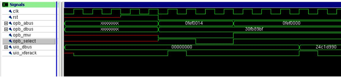
The amount of time taken for computation is seven cycles, which is the same as mode one. This is because mode one and mode two share the same functional units and data path in order to reduce area.
