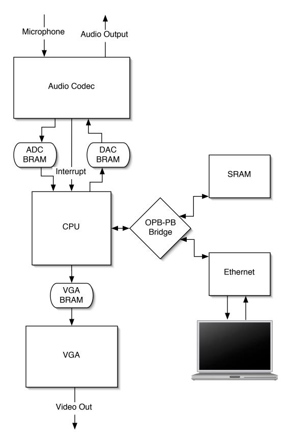
Figure 4: Implementation of Karaoke Machine Using Ethernet
