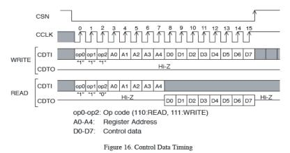
Figure 6: The timing diagram for writing to a control register.
