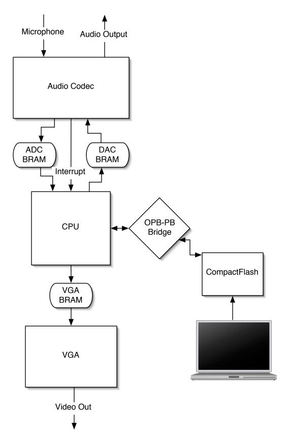
Figure 2: Implementation of Karaoke Machine Using CompactFlash
