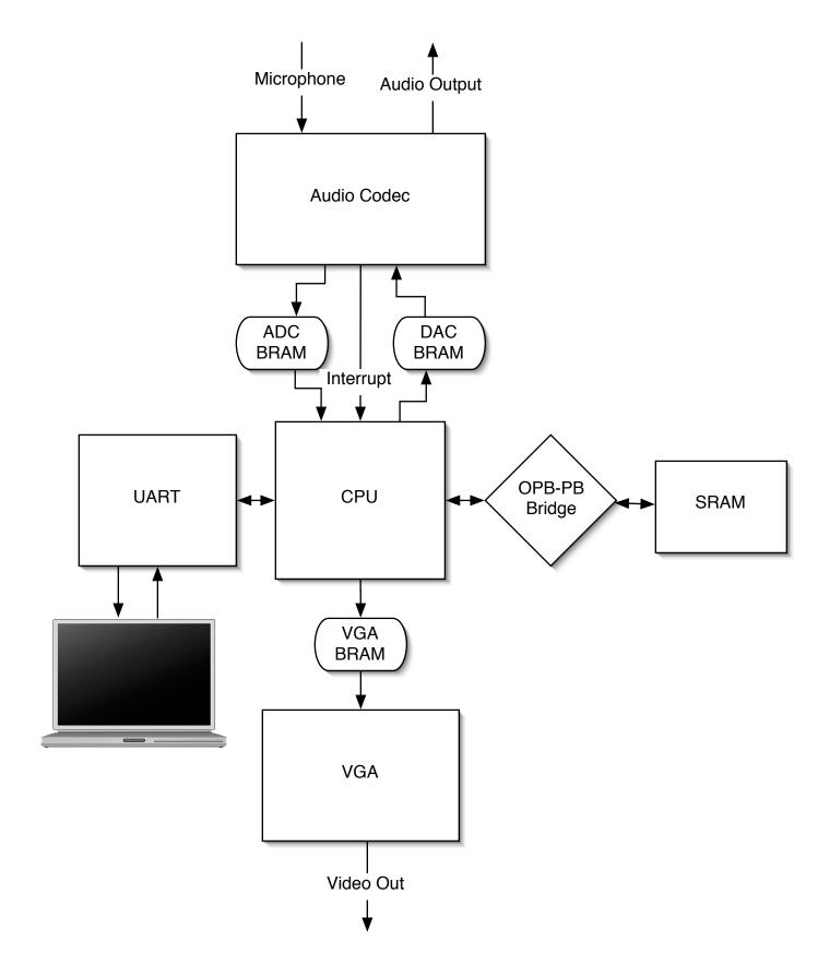
Figure 3: Implementation of Karaoke Machine Using UART
