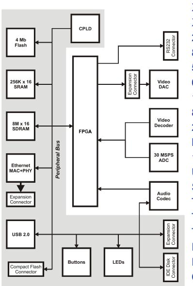
XC2S300E FPGA XC9572 CPLD 256K x 16 SRAM 8M x 16 SDRAM 512K x 8 Flash 6-channel NTSC video decoder 12-bit, 30 MSPS ADC 80 MHz, 30-bit video DAC 20-bit, 4-input, 1-output stereo codec Microphone/line-in/line-out jacks 10/100 Fthernet MAC+PHY USB 2.0 peripheral port Six pushbuttons, DIP switch Two LED digits, bargraph Three programmable oscillators Two expansion headers w/ 75 I/O pins Peripheral header w/ 18 I/O pins Parallel and Serial port Compact Flash interface
