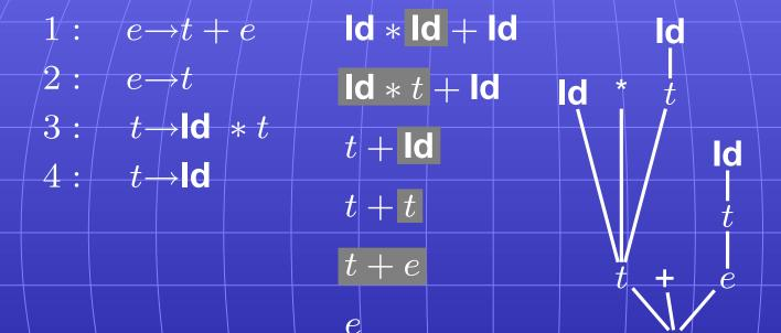
This is a reverse rightmost derivation for **Id** \* **Id** + **Id**. Each highlighted section is a handle. Taken in order, the handles build the tree from the leaves to the root.
