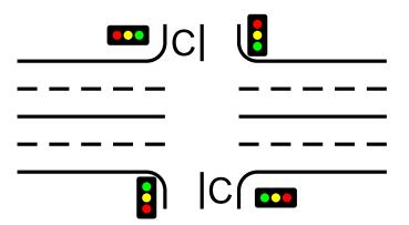
This controls a traffic light at the intersection of a busy highway and a farm road. Normally, the highway light is green but if a sensor detects a car on the farm
