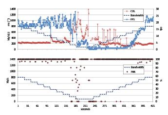
*Figure 3:* CDL, fps, and FRR for Skype as a function of time when the available bandwidth is adjusted as a step function.
