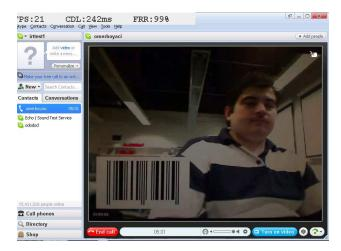
*Figure 2:* Screen shot of the receiver side vDelay application. FPS, CDL, and FRR statistics are shown at the top of the image. The barcode received from the caller user agent is also visible.
