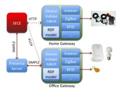
Fig. 3. The architecture of sensors and actuators gateway
