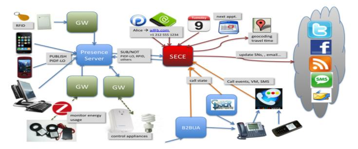
Fig. 2. The Architecture of SECE
