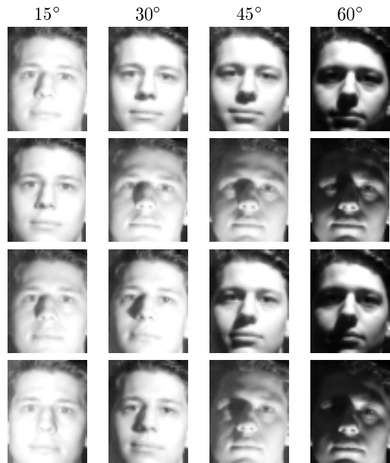
Figure 1: Pictures from the Harvard Face Database. The pictures are of the same individual lit by varying the direction of a point light source. The angle of the light source with the optical axis (15, 30, 45, and 60 degrees) is the same in each column.
