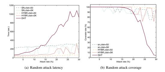
**Fig. 2.** Figures (a) and (b) illustrate the latency and coverage for the random attack scenario respectively and for different attack intensities. In (a), Y-axis shows average notification time and in (b), Y-axis shows the percentage of nodes which successfully received the alert message.
