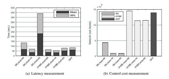
**Fig. 1.** The evaluation results under normal operations. Figure (a) depicts the mean notification time and the completion time for 99% of the nodes and for different control plane mechanisms. Figure (b) presents the total network cost in terms of bytes for the test duration of 600 seconds.
