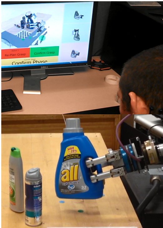
Fig. 5: Above is the subject confirming a grasp for the handle of the detergent bottle at the RASCAL lab. Below is the realized grasp of the successfully lifted detergent bottle at Columbia University.
